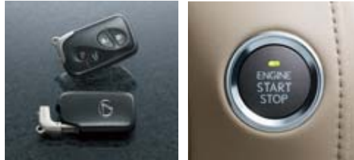
The smart key fob can remain in your pocket. LX570 will recognise you as the driver and release door locks when you lightly touch the door handle. An ultra-thin electronic card key is also provided that slips easily into your wallet alongside credit cards.
