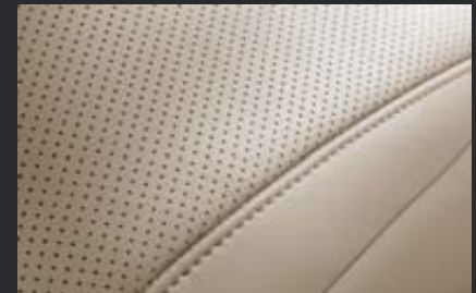
Fine perforations in the driver and front passenger seat cushions allow cooling air to maintain comfort.
