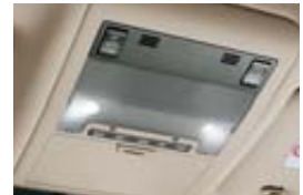
LED spots provide night time spot illumination for front seat occupants.
