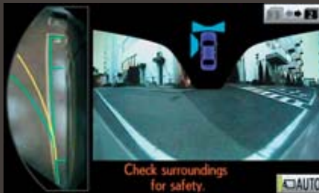
Wide-view front and side monitor system display screen
