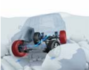
Crawl Control manages braking and acceleration when LX570 is negotiating rough terrain or a steep descent.
