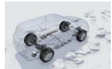
Four-wheel Active Height Control automatically adjusts ride height depending on vehicle speed.
