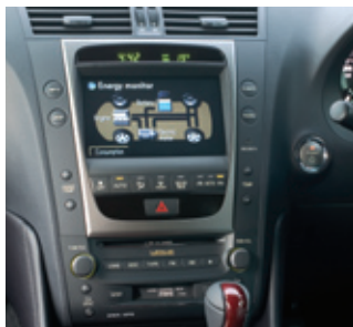
THE 7" ELECTRO MULTI-VISION (EMV) DISPLAY IN THE CENTRE CONSOLE OF GS450h DISPLAYS FUEL CONSUMPTION IN REAL TIME AND AN ENERGY MONITOR WHICH SHOWS THE FLOW OF ENERGY BETWEEN THE PETROL ENGINE, ELECTRIC MOTOR, THE BATTERY AND REAR WHEELS SO YOU CAN SEE THE INNOVATIVE HYBRID SYSTEM IN ACTION.
