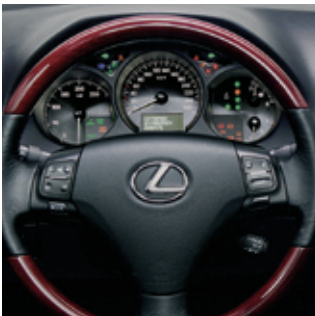
INSTEAD OF A TYPICAL REV COUNTER, THE GS450h IS FITTED WITH A SPECIALLY DESIGNED ENERGY MONITOR TO MEASURE POWER FLOW IN KILOWATTS AND THE AMOUNT OF ENERGY BEING REGENERATED FROM THE WHEELS.
